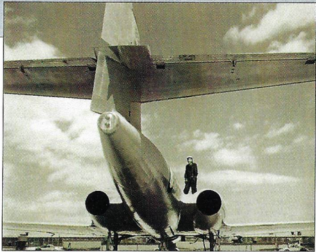
Above: The twin Canadian-built Orenda turbojets were non-afterburning units, but provided a useful amount of thrust as well as fuel efficiency and reliability for long-range patrol missions.
