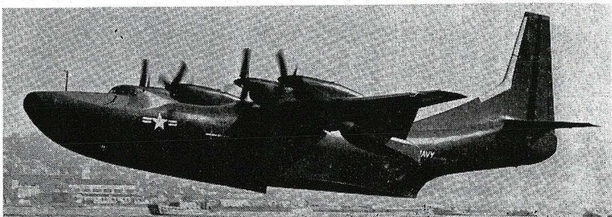
THE CONVAIR R3Y TRADEWIND TRANSPORT—America's first turboprop seaplane takes off on San Diego Bay for its maiden flight. The 80-ton high-speed transport took off in less than 30 seconds and remained in the air during a shakedown test program for more than two hours.
