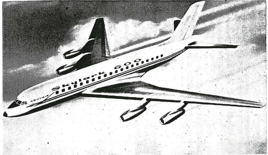
CONVAIR'S jet transport proposal for a medium range jet airliner. The Skylark 600, says Convairstar, will have a 609 mph cruising speed. On a first-class 80-passenger configuration operating costs will be 1.4c to 1.7c per seat mile. Over a 500-mile range block speed will be 413 mph, on a 1,000-mile stage the speed will be 470 mph and 504 mph block speed on a 1,500-mile stage. The engines will be General Electric CJ-805's—commercial version of the J79.
