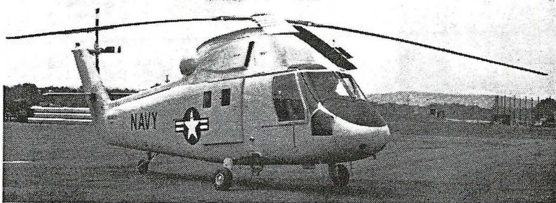
KAMAN HU2K-1 HELICOPTER: Above is a full scale mock-up of the U.S. Navy's HU2K-1 utility helicopter. Winner of a Navy design competition, the HU2K-1 will be powered by a General Electric T-58 gas turbine, shown below. Engine weighs 325 lbs., is 59 inches long, 16 inches in diameter. Preliminary tests reveal that T-58 engine produces 1065 horsepower.
