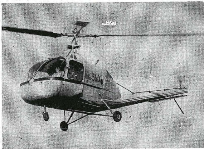
Shown on a test flight three days after coming out of the shop, the Hiller "360" displays the simple pattern of its design. The pilot and two passengers sit abreast in the wide cabin quite comfortably. Production models will have a fairing over the tail rotor drive shaft.
