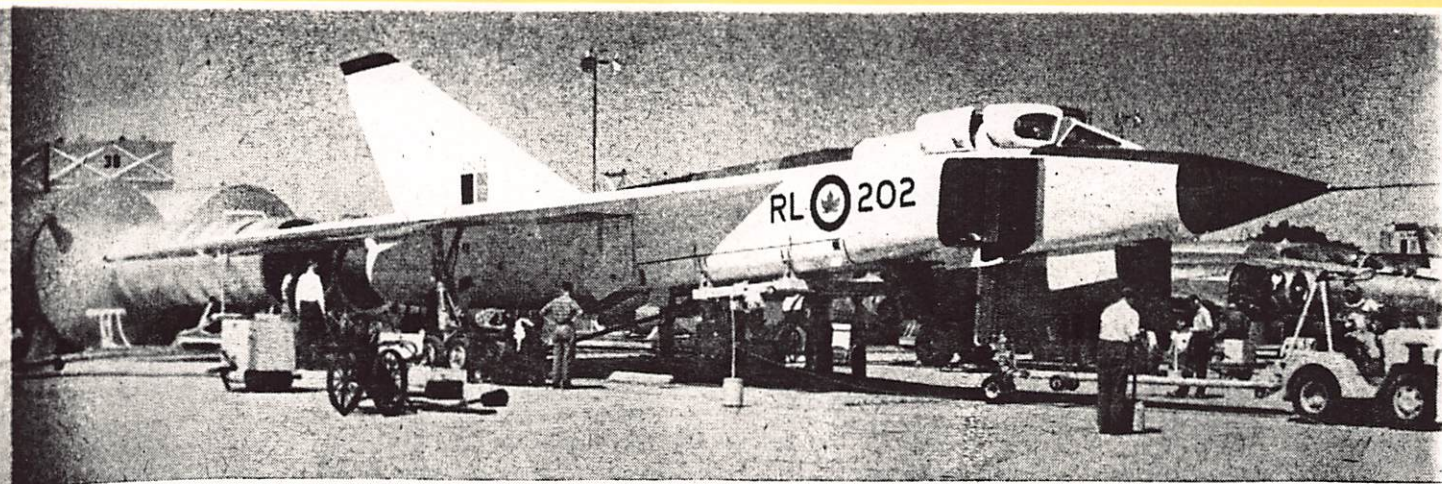
The second Arrow undergoing engine runs—with noise suppressors—at Malton. A third has already flown.
