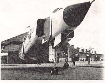
Above, the Arrow's fuse-lage is characterized by a "rectangular" cross-section to accommodate the side-by-side powerplants—which in the prototype are Pratt & Whitney J75s; production Arrows will have the Orenda Engines Iroquois turbojets. Left, the combined saw-tooth and "cut" in the leading-edge of the exceptionally thin 60 swept wing.
