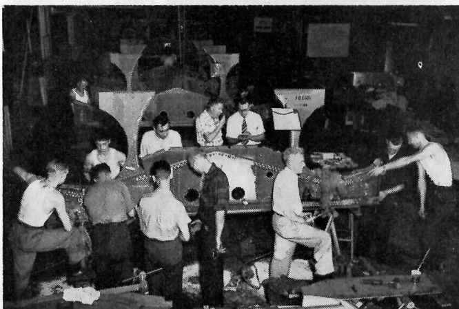
Production line final bolt-up of main spar of centre section, shimming root ends.
