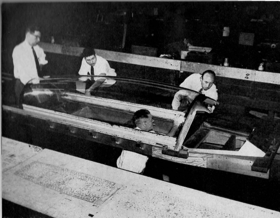
Planners checking canopy assembly subcontract unit with jig for trim tolerances.
