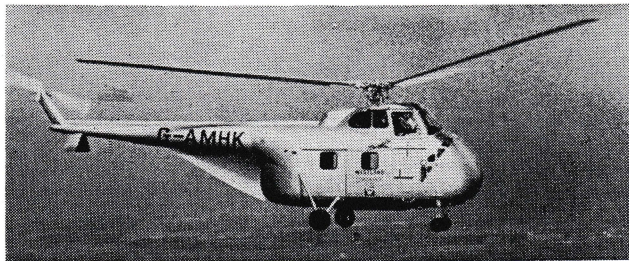
TO BE BUILT IN UK—The Sikorsky S.55 12-place helicopter which is to be built in the United Kingdom under license. It has a range of over 400 miles. Normal gross weight is 6,800 lb. Useful load is 2,400 lb. The smaller S.51, known as the Dragonfly in England, is now standard equipment on all Royal Navy carriers.
