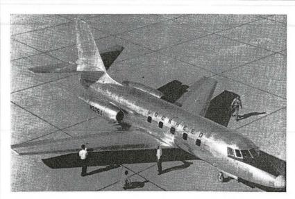
LOCKHEED JETSTAR: Seen above on the ramp, and below in flight for the first time, the Lockheed JetStar presents a study in speed. The 500-550 mph, 10-passenger utility jet transport is at Edwards AFB for flight tests. Pods on rear fuselage contain Bristol Orpheus engines, with take-off thrust totalling 10,000 lbs. The JetStar's 53-foot wing has a 34-degree sweep back on the leading edge.
