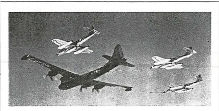
FEEDING TIME: This flight photo shows an actual triple-refueling operation being carried out with a USAF B-29 tanker aircraft and three RAF Gloster Meteors. Developed by the British company, Flight Refuelling Limited, the probe & drogue system has met with greater acceptance in the U.S. than in Britain. It is used by both the USAF and the USN. A number of other systems have been tried, but most lack the simplicity of Flight Refuelling's probe & drogue.
