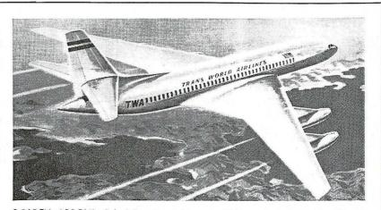
GOLDEN ARROW: Scheduled for delivery to TWA early in 1959, the Convair Golden Arrow medium range jet transport (above), will have a cruising speed of 609 mph and will be powered by four GE J-79/CJ-805 turbojets of approximately 15,000 lb. th. each. The Golden Arrow is ostensibly almost identical to the Skylark 600 announced earlier. Horizontal stabilizer is mounted on the fuselage of the Skylark; Golden Arrow is distinguished by its gold finish.
