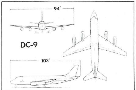
DOUGLAS DC-9 PROPOSED: An advanced short/medium range jet transport is being offered by the Douglas Aircraft Co. for operation in 1963. Powered by four P & W turbofan engines known as the Model JTF10A-1, the new aircraft will carry 68 first class or 92 coach class passengers over short to medium ranges at speeds and comfort comparable to the larger DC-8. The powerplant is being designed specially for the DC-9.
