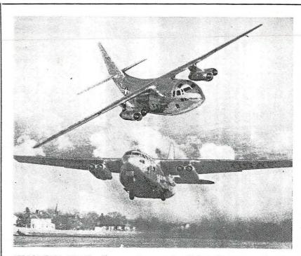
JET-POWERED CHASE: \_Shown on its recent first flight is this jet-powered version of the Chase Aircraft Company's C-123. Known as the XC-123A, this aircraft is powered by four General Electric J-47s and is a development of the version powered by two P & W R-2800s, which in turn was originally developed from the Chase CG-20 all-metal cargo glider. On its first flight the aircraft was off the ground in just over 1,000 feet and attained an estimated speed of more than 300 miles per hr.
