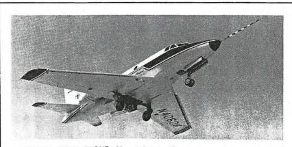
SABRELINER FIRST FLIGHT: New twin-jet utility trainer and transport, North American Sabreliner, is shown on its first flight, Sept. 16. Capable of carrying up to ten persons, Sabreliner has 15,330 lb. gross weight. Powered by two GE J-85 turbojets, the transport cruises at 500 mph at 45,000 ft., with cabin pressurized at 8000 ft. Length, 43 ft.; span, 42 ft.; height, 16 ft.
