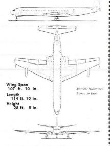
operation, though with some loss in maximum range. In addition, for structural reasons the fastest cruising altitude in the case of the 4 will be higher by some 5,000 ft. and the cruising speed somewhat lower as compared with the 4A. Similarly, the 4A could be operated using the normal long-range technique, but its longest practical stage length would be somewhat less than that of the 4.
