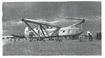
Powered by a Rolls-Royce Merlin, the Cierva W.II Air Horse must be the largest helicopter at present flying. It carries 24 passengers or three tons.
