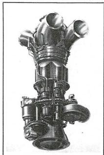
NAPIER GAZELLE JUNIOR: New free turbine engine by D. Napier & Sons, available both for helicopter application and as a propeller turbine. Initiall rating is 920 shp, but this will be increased to 1,070 shp during development.
