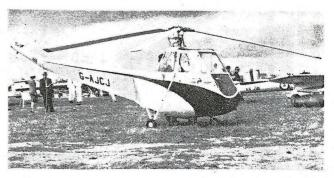
The Cierva W.14 Skeeter has been designed as a two-seat trainer or passenger autogyro. It is powered by a 106 hp Jameson F.F.I. engine.
