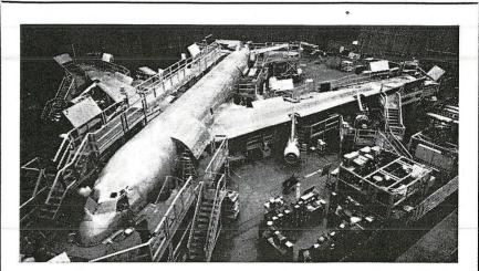
BOEING MEANS BUSINESS: A private investment of \$15,000,000 is represented by this jet transport, shown in an advanced state of prototype construction at the plant of Boeing Airplane Co., Seattle, Wash. Powered by four P & W J-57's, the Boeing transport has an all-up weight of 190,000 lbs., a span of 130 ft., and length of 128 ft. Design cruising speed is 550 mph, while capacity will be between 80 and 150 passengers. Model below shows how completed aircraft will appear.
