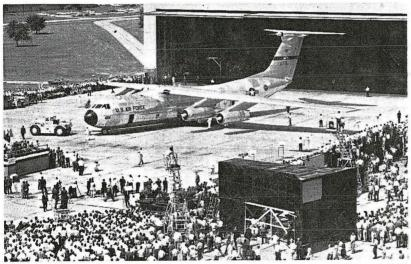
ROLL OUT of the Lockheed C-141A Starlifter, designed for military and civil operation. Span of the aircraft is 160 ft; power is provided by four P & W fan-jets giving a total of 84,000 lb of thrust.
