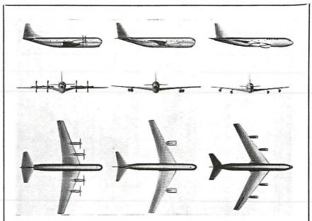
EVOLUTION OF A JET TRANSPORT: Models illustrate some of the stages through which Boeing design studies led when considering layouts for gas turbine powered transports. Left is the Model 367-60, a gull-wing, turboprop design which utilized the C-97 fuselage and empennage; centre is Model 367-64, which also used the C-97 fuselage. It featured pod-mounted turbojets, swept wings and tail surfaces. Right is the final choice, the Boeing Stratoliner, soon to fly.
