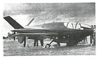
Of magnesium construction the novel Planet Satellite is intended for the personal plane market. Engine is located just behind passenger cabin.
