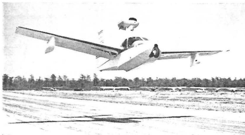
SKIMMER AMPHIBIAN: Lund Aviation (Canada) Ltd. has recently been appointed Canadian distributor for Colonial Aircraft Corp.'s Skimmer, a 3-place amphibian. Powered by a 150 hp Lycoming engine the aircraft has an all-up weight of 2,150 pounds and a range of 700 miles. Wing span is 34 feet; length 23 ft. 6 in.; and height 8 ft. 10 inches. Maximum rated speed for the Skimmer is 127 mph, while landing speed is 50 mph. The main landing gear folds into the wings while the nose wheel retracts forward into the fuselage.
