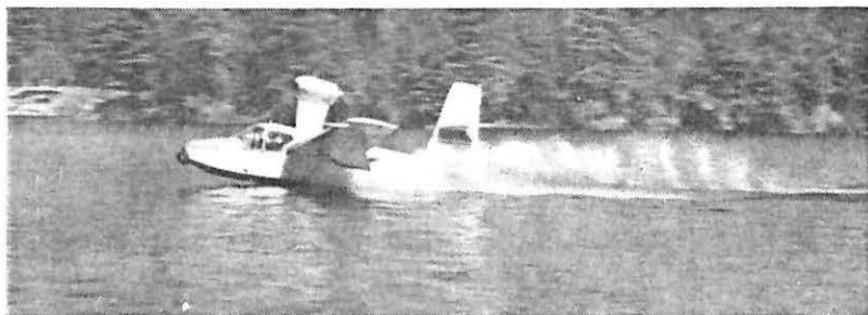
SKIMMER AMPHIBIAN: Lund Aviation (Canada) Ltd. has recently been appointed Canadian distributor for Colonial Aircraft Corp.'s Skimmer, a 3-place amphibian. Powered by a 150 hp Lycoming engine the aircraft has an all-up weight of 2,150 pounds and a range of 700 miles. Wing span is 34 feet; length 23 ft. 6 in.; and height 8 ft. 10 inches. Maximum rated speed for the Skimmer is 127 mph, while landing speed is 50 mph. The main landing gear folds into the wings while the nose wheel retracts forward into the fuselage.
