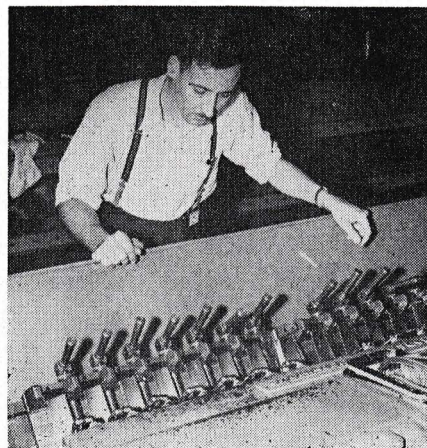
View from above and rear of Avro Canada's new Tracermatic 14-Spindle Duplicator for making gas turbine blades.
