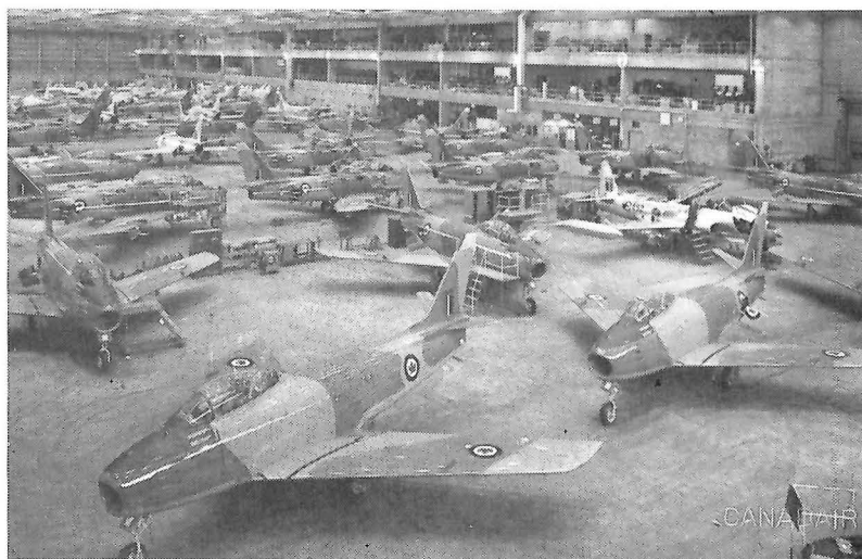
COLORFUL SABRES: Crowded with Sabre 6's and T-33's is Canadair's big flight test hangar. Sabres wear the new camouflage scheme in which all aircraft of this type are now being finished. Scheme utilizes two shades of green on upper surfaces, and light blue underwing and belly. RCAF Sabres in Europe have flatter finish than evident above and also have Canadian ensign in place of the tri-color bar on the vertical fin. No squadron insignia are being permitted.
