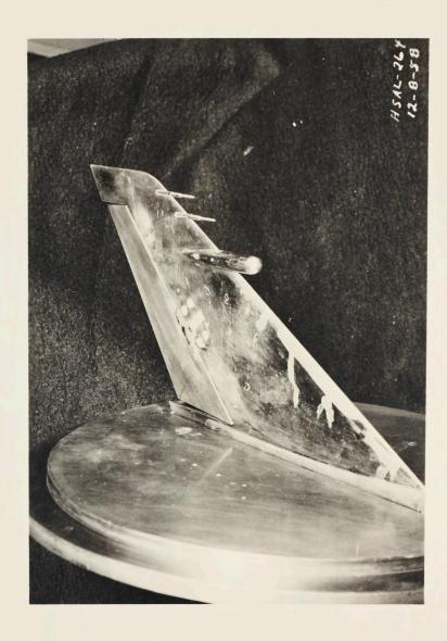
Fig. 1 The .04 Scale Arrow (C-105) Vertical Tail
