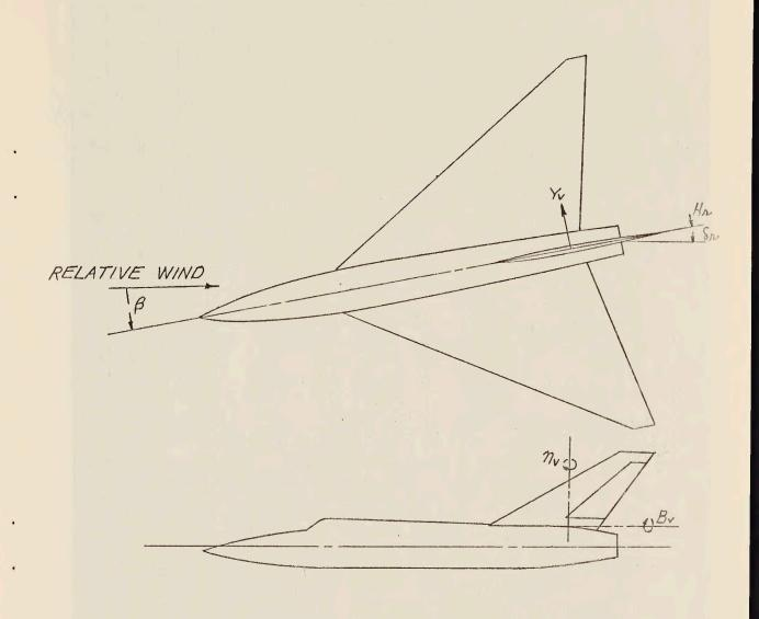
FIG. 3- SYSTEM OF AXES
