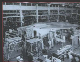
The first inner wing now assembled to the first fuselage.
