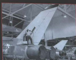
Mechanics looking into tail of Avro Arrow RL25203. Note size of jet pipes, RL25202 is parked behind.
