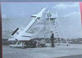
Final adjustments being made ready to launch Free Flight model No. 8 on a Nike rocket booster
