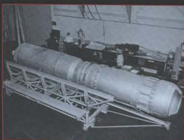
Mock up of a Pratt & Whitney J75 engine used for installation tests.
