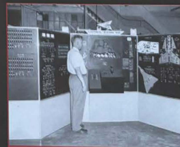
The electrical system test panel can simulate the Arrow electrical system and test any installed components.
