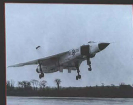
Avro Arrow RL25201 landing after its first test flight. Note the dive brakes are deployed.
