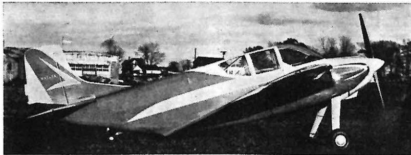
PARAPLANE COMMUTER 110: With a two-place conversion underway (the 120), the recently developed Paraplane Commuter 110 is a low-cost ultra-safe business aircraft designed for plant-to-plant flight operations, parts delivery and sales work. It will hover at 15 mph or cruise at 165 mph.; can be landed onto and flown out of areas previously restricted to helicopters.
