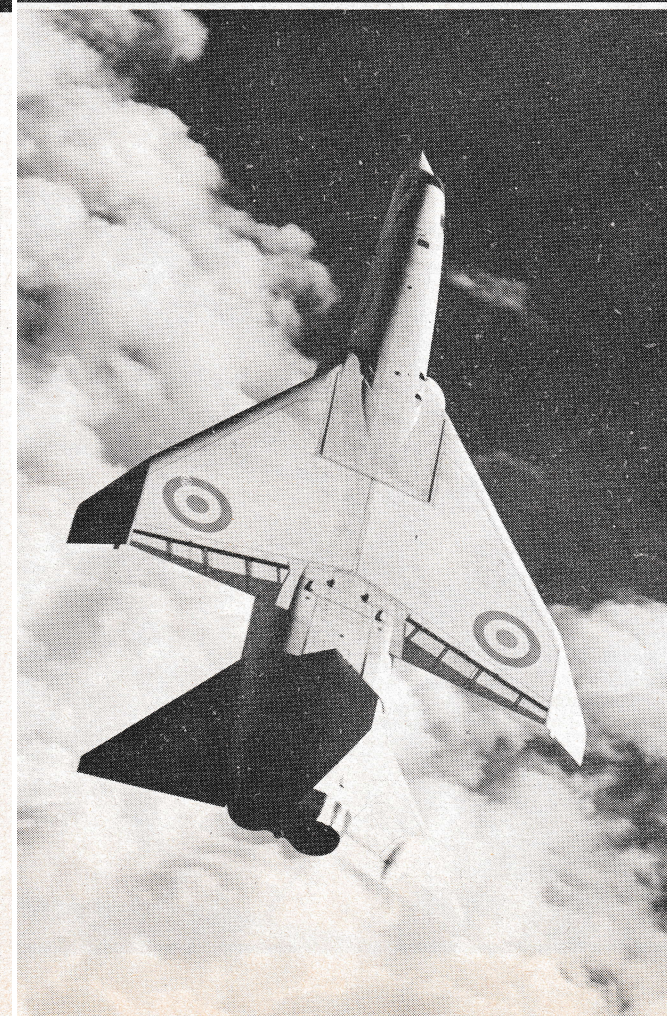
Above, the first prototype TSR-2 lets it all hang out. Full-span blown flaps gave good short-field performance. Below, welders cut up the 750-million-dollar machine for scrap. The carcass ended life as a gunnery target.
