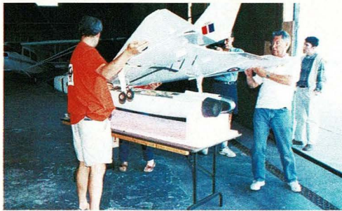
The model Avro Arrows were constructed in a modular fashion. Here production supervisor Time Bider (left) and Jerry Fingler (right), model maker assemble one of the models for a test flight.
