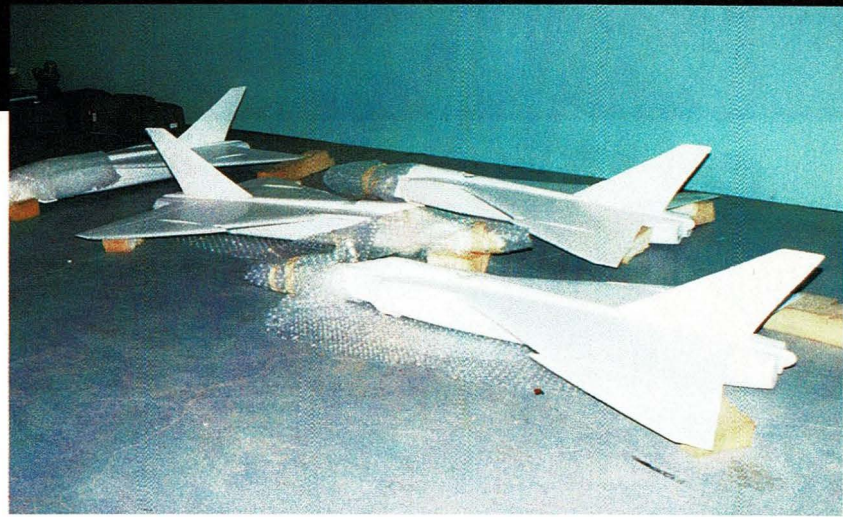
Many scale models were constructed- this group was used to portray the real life" scale models that were launched from a Nike rocket.
