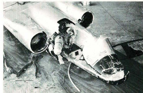
Rough landings and problems with the ducted fan engines of the RC models slowed the F/X filming.
