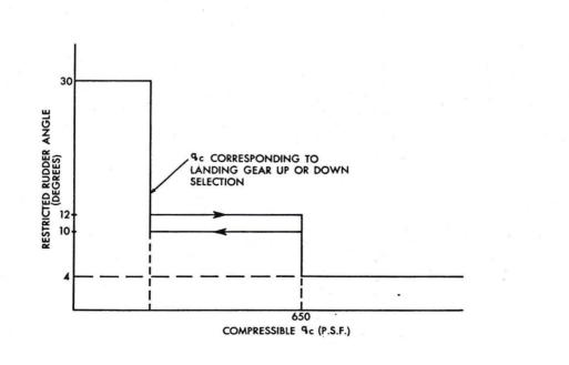
FIG. 21 Qc ACTUATOR SYSTEM - CHARACTERISTICS
