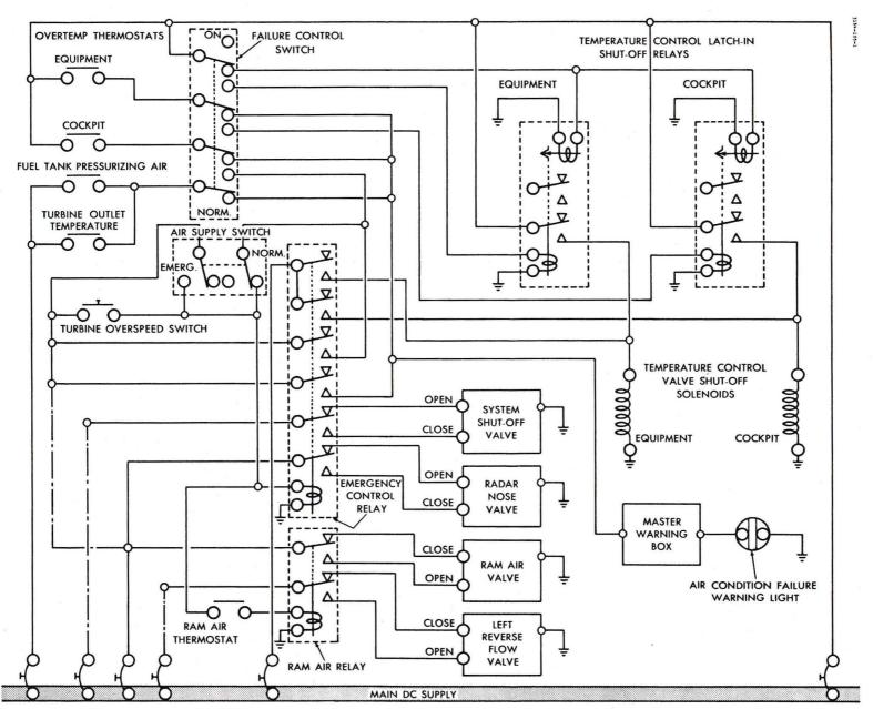
FIG. 12 ARROW 2 AIR CONDITIONING FAILURE PROTECTION
