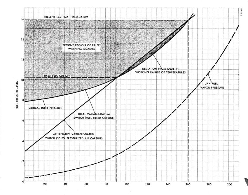
FIG. 15 FUEL PRESSURE WARNING SWITCH CHARACTERISTICS
