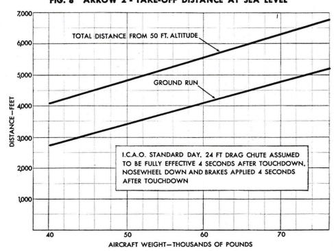
FIG. 9 ARROW 2 - LANDING DISTANCE AT SEA LEVEL
