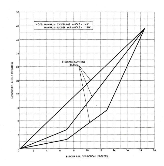
FIG. 17 NOSEWHEEL STEERING CONTROL CHARACTERISTICS (TRIAL INSTALLATION)
