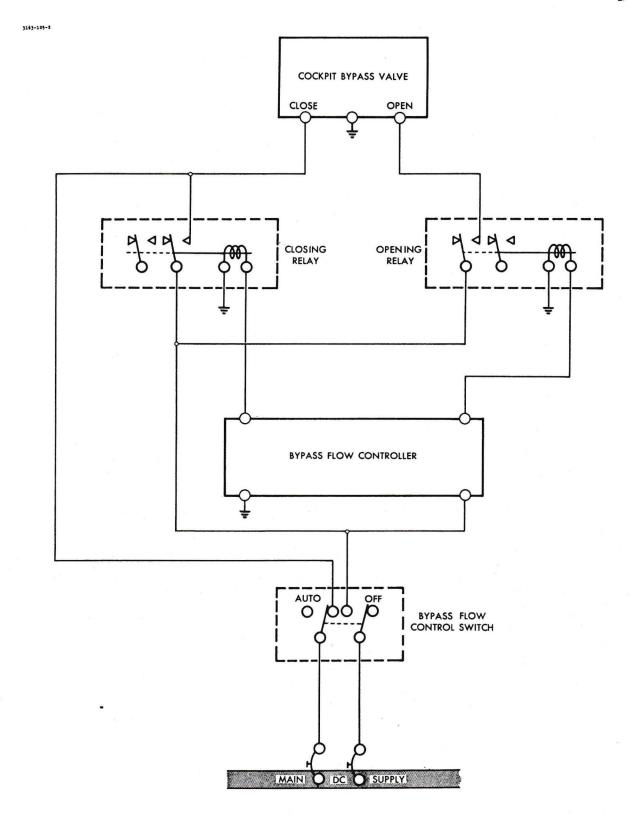
FIG. 11 COCKPIT BYPASS FLOW CONTROL SYSTEM - ARROW 2 (TRIAL INSTALLATION)
