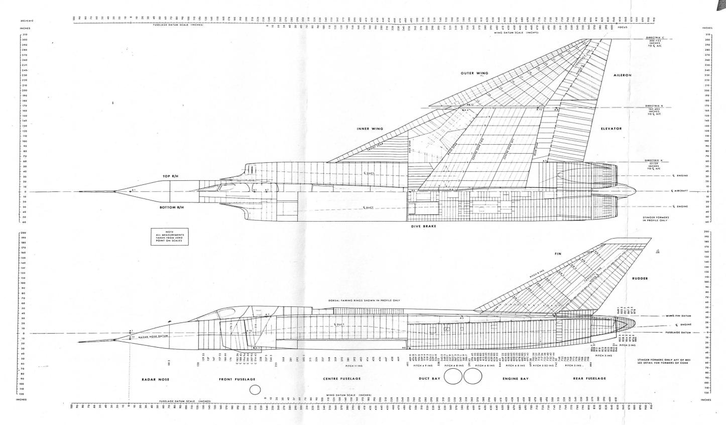
FIG. 23 ARROW STATION AND DATUM LINES
