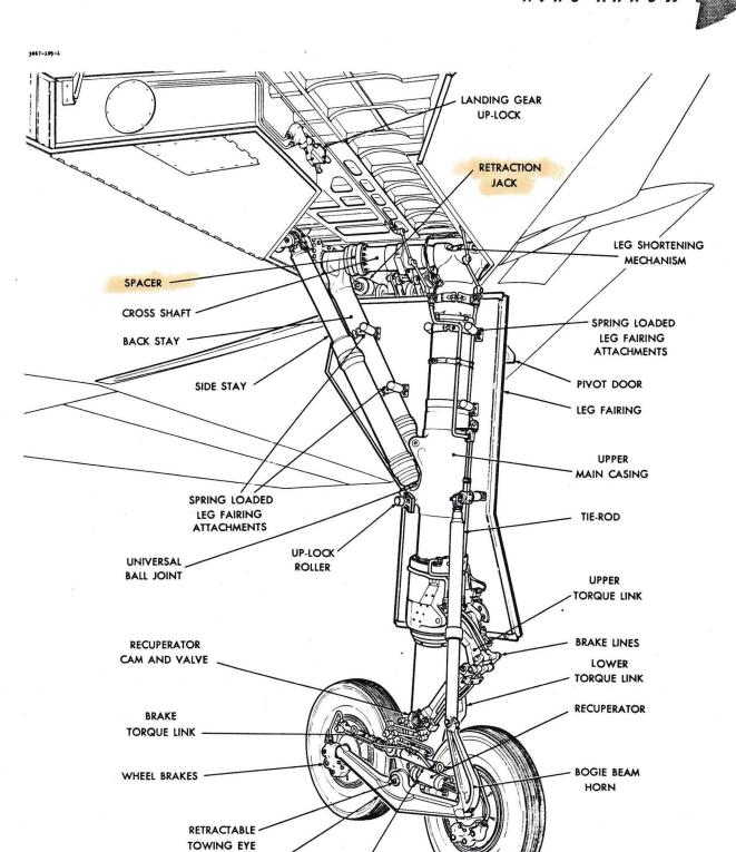
FIG. 24 LEFT-HAND MAIN LANDING GEAR ASSEMBLY
