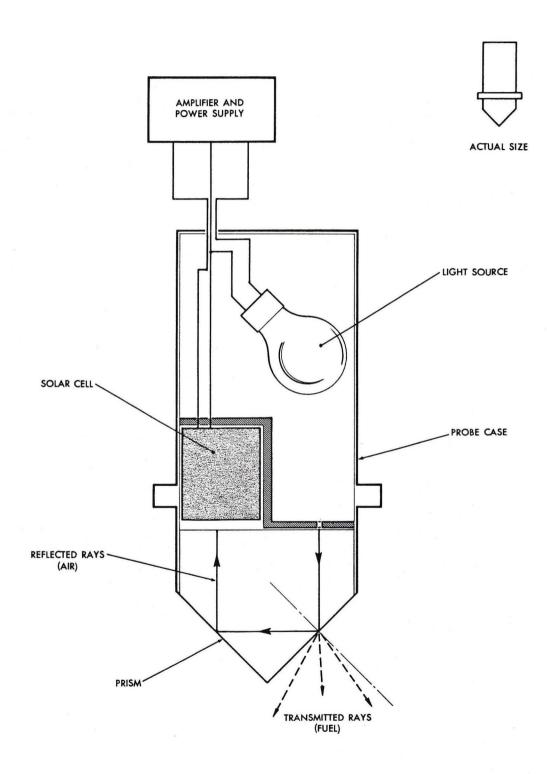
FIG. 16 OPTICAL SENSING PROBE
