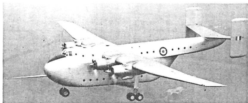
FRONT AND BACK: The Blackburn Beverly prototype is shown on its recent first flight. The aircraft is the forerunner of the Beverly C. Mk. I transport which is being produced in quantity for the RAF. The Beverly can carry, simultaneously, ten jeeps and 42 troops. Powered by four Bristol Centaurus engines, the aircraft has a span of 162 feet, a length of 99 feet, and a height of 38 feet.
