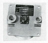
A force-balance direct-acting mach switch, claimed to provide a weight saving of as much as two pounds (above) is announced by **Burton Manufacturing Co.**, Santa Monica, Calif. The unit is about 4 in. in diameter and 1½ in. in depth. Weight is 1 lb. Instrument is claimed to provide an accuracy of plus or minus 2 percent with an altitude range to 70,000 feet. It can be made to open or close at selected mach points up to 2 mach.
