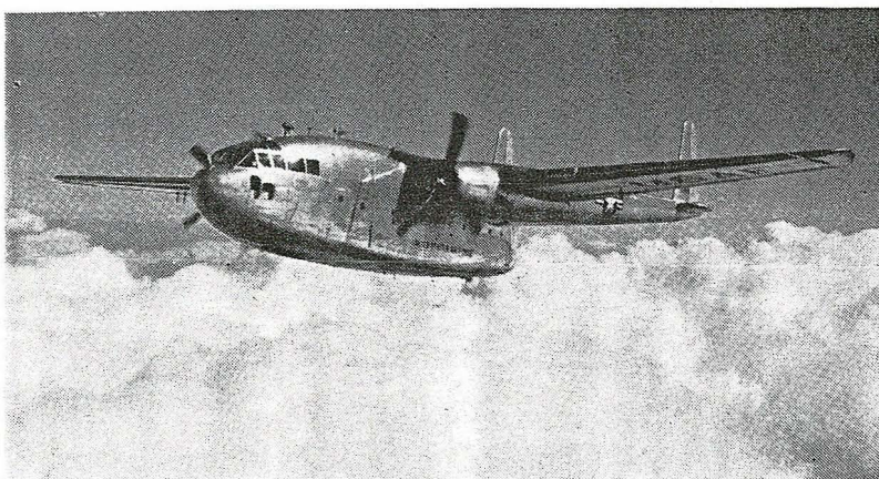
PACKAGED GOODS: The new Fairchild C-119 Packet is shown. The Packet has been designed as a replacement for the C-82. The C-119 has greater speed, payload and range than the older type aircraft and can carry 42 fully armed paratroopers, as well as twenty 500-pound containers of supplies. Alternatively it can carry ten tons of cargo. USAF and USN orders for C-119's at present total 143.
