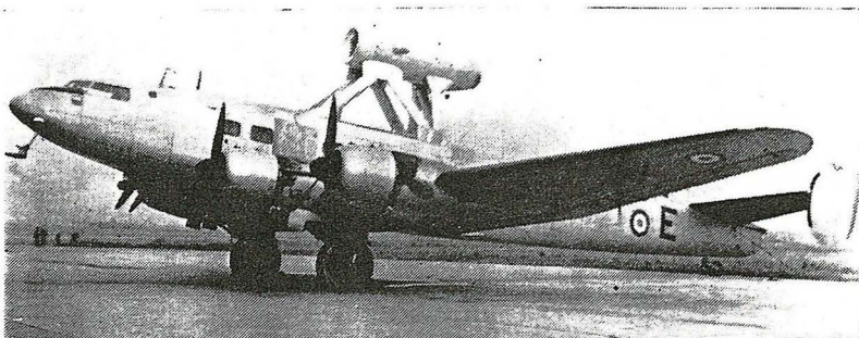
PICK-A-BACK: Since the War, France has produced an unusual variety of new airframe and engine designs. Above is the now well known Languedoc, widely used by Air France and French Air Force. This one is being used as a flying test bed for the new Snecma Atar 101 turbojet.
