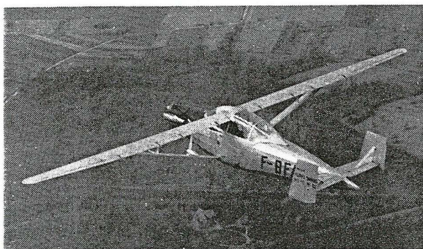
LONG AND LEAN: Immediately above is the experimental Hurel-Dubois HD.10 aircraft with high aspect ratio wing. At right, a proposed SNASCO medium jetliner which would be powered by Avons, Sapphires, or Atars.
