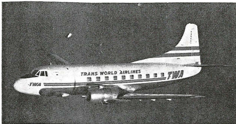
FIRST FLIGHT: Shown on its first flight is the new Martin 4-0-4, 103 of which are on order, including 60 for Eastern Air Lines and 40 for Trans World Airlines. The 4-0-4 is an enlarged and improved version of the 2-0-2. The aircraft carries forty passengers in a pressurized cabin and is powered by two Pratt & Whitney R-2800s.
