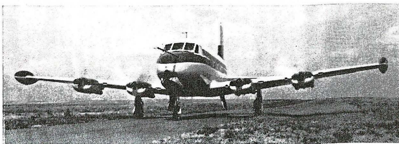
CESSNA 620 AIRBORNE: On August 11, Cessna Aircraft Co.'s, new Model 620 successfully made its maiden flight, remaining in the air for about 45 minutes. Cessna describes the 620 as being the world's first four-engine, pressurized airplane to be developed for the executive transport market. The engines are Continental GSO-526-A's, each developing 320 hp for take-off. Design cruising speed is 235 mph @ 18,000 feet.
