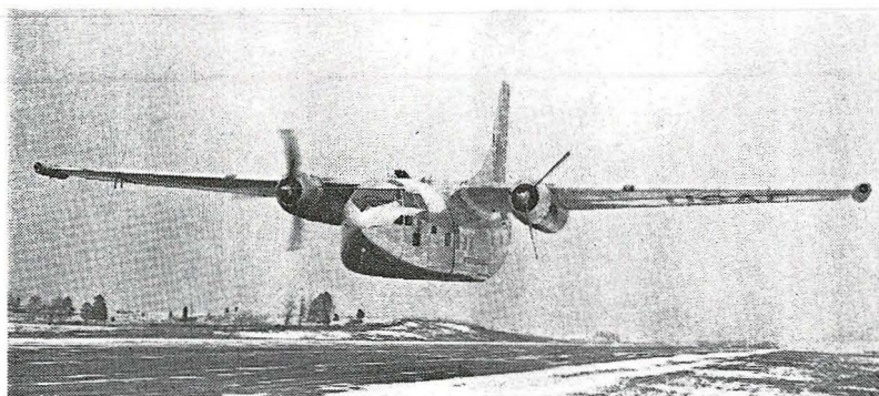
TRANSPORT TRICKS: Fairchild C-123B transport experimentally fitted with wing-tip-mounted Fairchild J-44 turbojets of 1,000 lbs. th. each for thrust augmentation, is shown above making a low level flypast with one propeller feathered. Performance is described as "spectacular". Below, the Lockheed C-130 Hercules is shown flying by in "aerial delivery configuration" with rear ramp and door in open position, thus exposing the entire 9 ft. by 10 ft. cross section of the cargo compartment.
