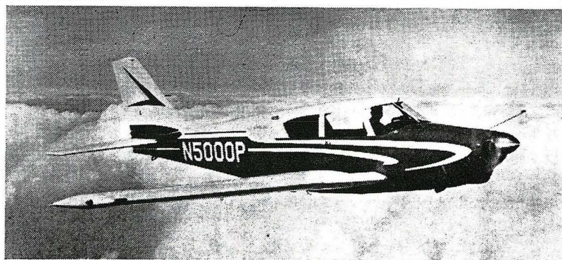
FIRST PRODUCTION COMMANCHE: First production model of the four-place Piper Commanche is shown here in flight. Production target is one per day in January, 1958, with an eventual goal of five per day. With 180 hp Lycoming, the Commanche cruises at 160 mph at 75% power at optimum altitude.
