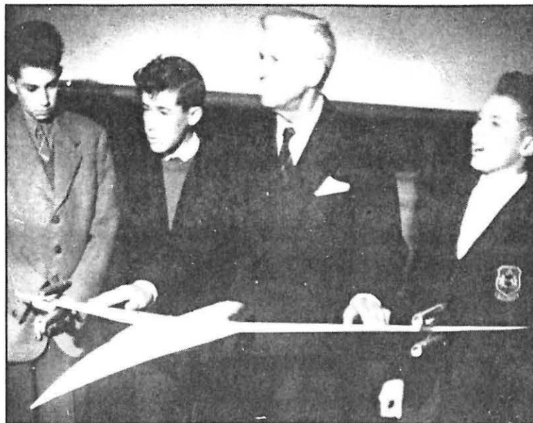
Above, Dr. Wallis is shown explaining the Swallow, with wings in subsonic position, to some of his audience; below, supersonic configuration.
