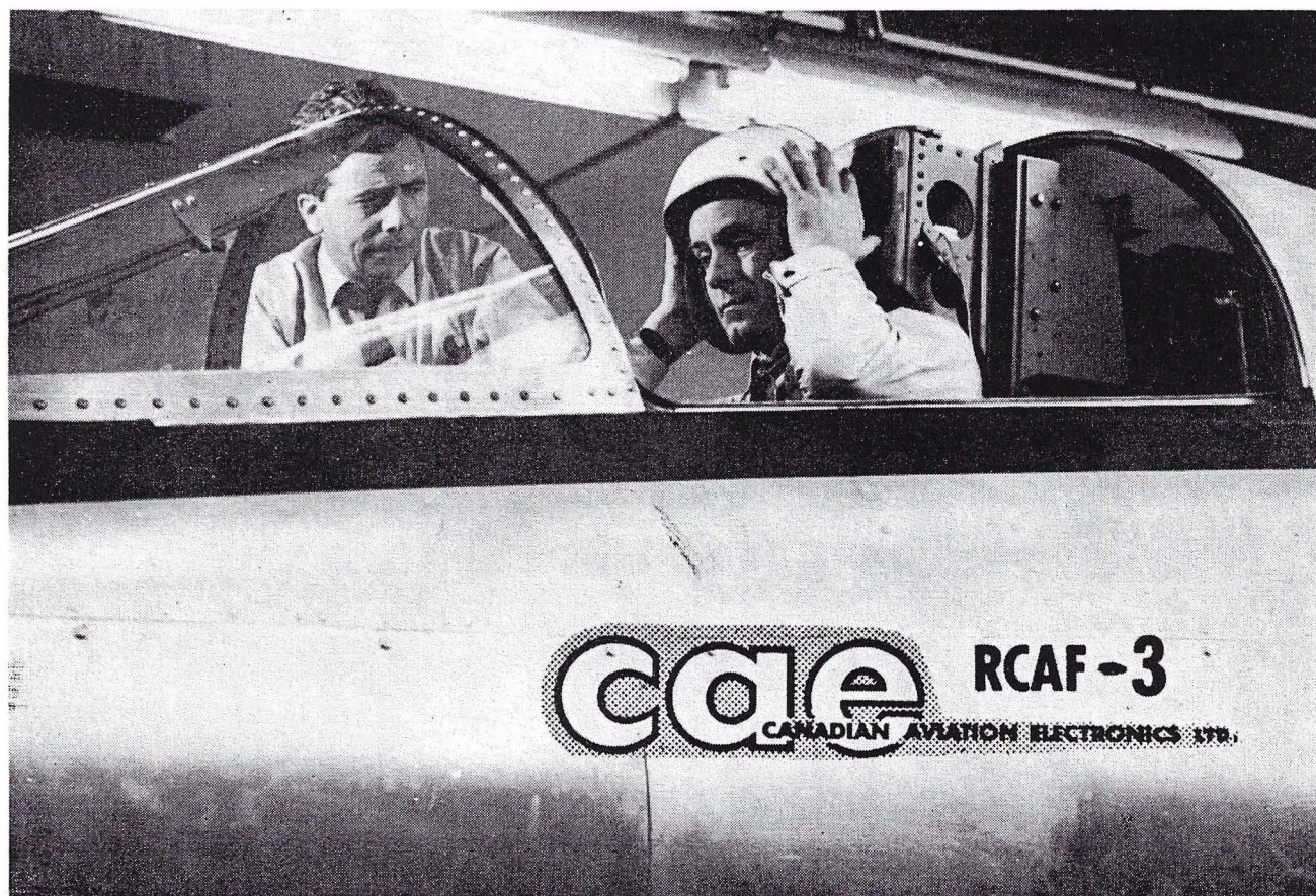
Representatives of the RCAF's IAM check out the crew compartment motion system of Canadian Aviation Electronics' CF-104 simulator which, along with F-104G simulator, is being produced for the RCAF and several NATO countries.
