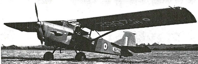
SIGHTSEEING: Latest version of the Auster AOP is the Mk. 9, which bears only a fleeting resemblance to its forebears: Powered by a 180 hp Blackburn Bombardier driving a Fairey fixed-pitch metal propeller, the Mk. 9 flies at a normal operational weight of about 2,100 lbs., at which weight it has a maximum cruising speed of 110 mph. In a 6 mph. wind it breaks ground in 325 ft.
