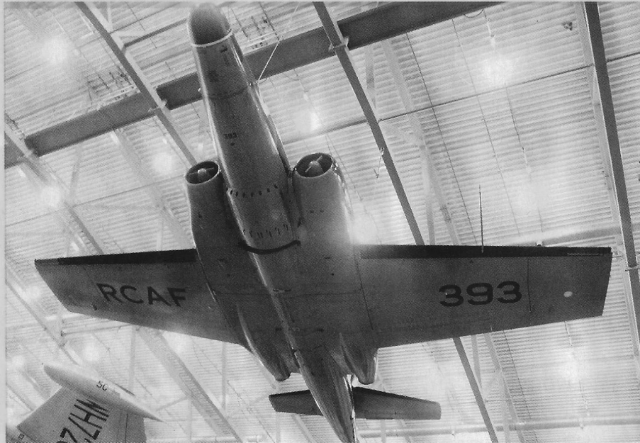
A unique view of the Avro Canada CF-100 Mk 4 from The Imperial War Museum at Duxford, England. It was Canada's main all-weather fighter of the 1950s, and the first combat aircraft of all-Canadian origin. The aircraft has a 53.5-foot wingspan and is 54 feet long with a service ceiling of 45,000 feet, and a top speed of 640 mph. This aircraft was built in 1955, and spent a large part of its operational life at Zweibrücken, Germany...a base I know well!
