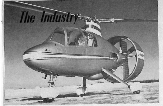
LATEST AVIAN 2/180 GYROPLANE appears in production form; modifications to be incorporated will not affect outward appearance to any degree. At present, Avian is building three more aircraft for use in final stages of the certification program, expected to be completed this summer.
