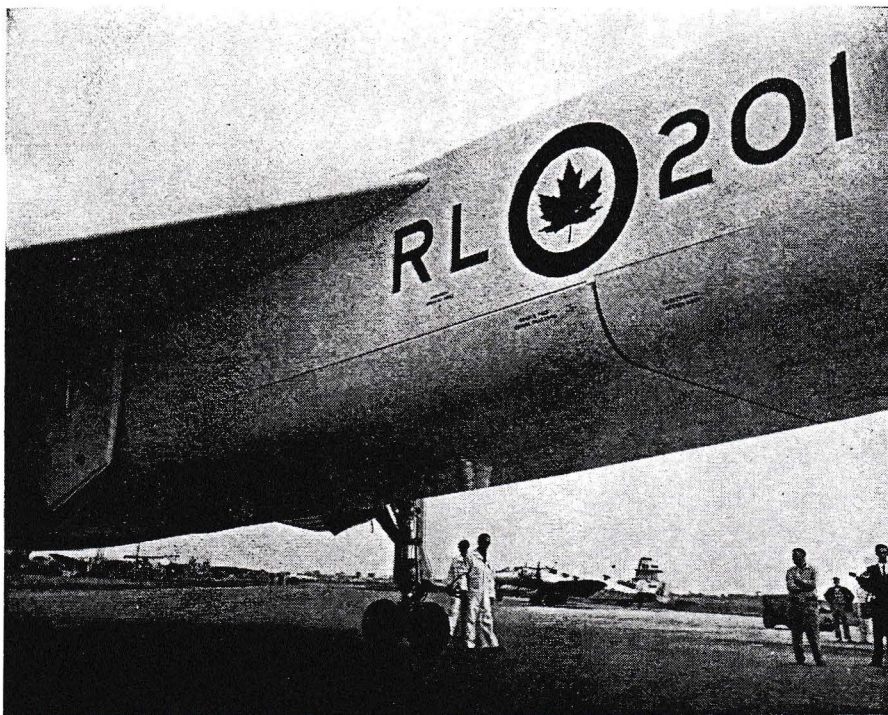
LARGE WEAPON BAY on the Arrow begins just under the RCAF roundel and runs aft to the landing gear door. The complete bay is removable to cut rearming time to a minimum. The bay carries air-to-air missiles with internal guidance.
