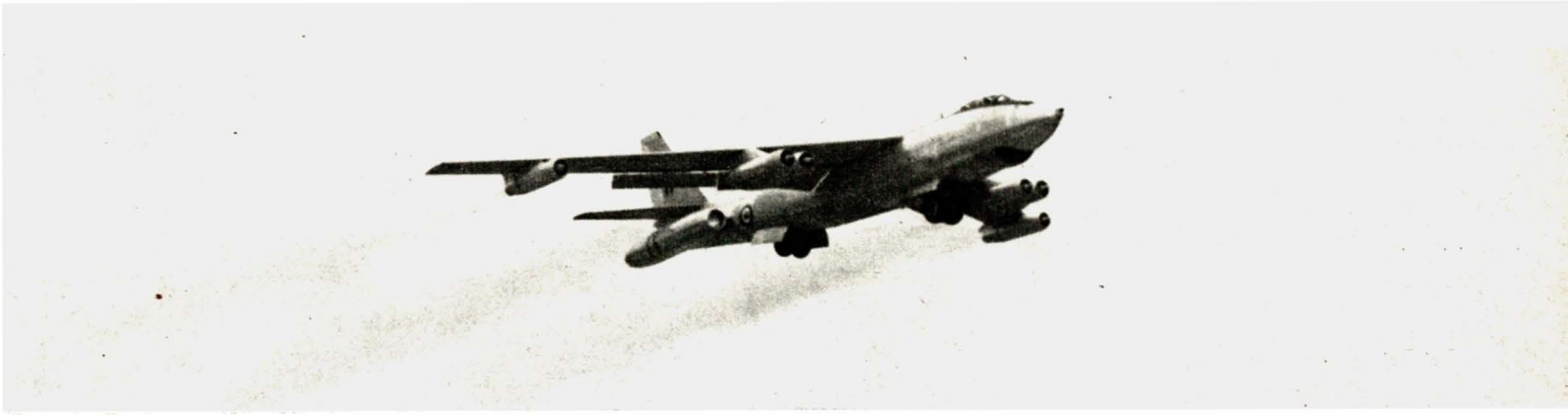
HOW IT FLEW: Fastened to the tail of a B-47 bomber, the Iroquois engine is test-flown near Toronto. Some experts believe, full out, its scream could kill.
