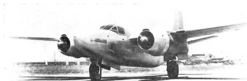
DOUGLAS B-26 CONVERSIONS: Above is seen the Lockheed Super 26, said to be the only pressurized B-26 offered today with an elongated fuselage and performance equal to or better than the wartime configuration. Below: the Silver Sixty, by the Rhodes Berry Co., of Los Angeles. This reasonably priced executive transport carries 14 passengers, 400 lbs. baggage, cruises at plus 300 mph.
