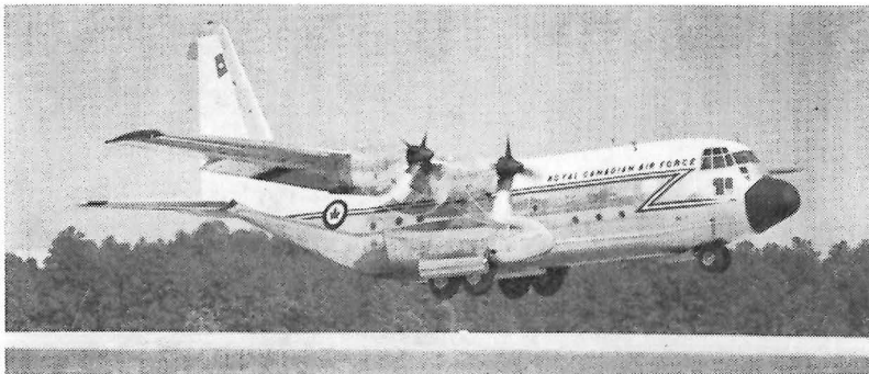
FIRST RCAF HERCULES: Deliveries of the RCAF's Lockheed C-130 Hercules transports began October 28. Powered by four Allison T-56 turboprops driving Aero-products propellers, the 124,200 lb. (max. gross) Hercules can carry a 15-ton cargo. The Hercules are being assigned to 435 Squadron at Edmonton. Although only four Hercules were ordered for the RCAF initially, it is understood that the number may be increased shortly.
