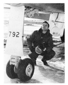
PRE FLIGHT CHECK of 792 last CF-100 to roll off Avro's production line is made by Chief Production Pilot Chris Pike prior to taking the airplane into the air for the first time recently for a production flight test. All pilots personally check each airplane visually from the ground before climbing into the cockpit for further checks before taxing out to take off.
