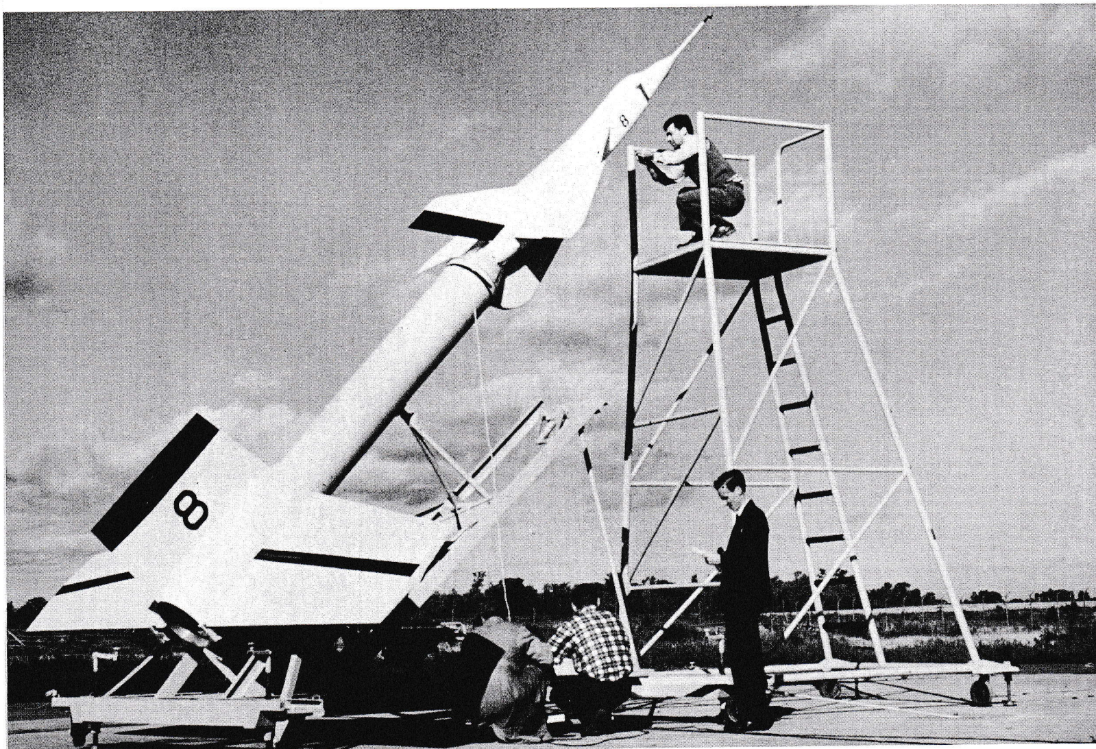
At altitude, the free-flight model is loosed from the Nike. Instruments send to the ground information on the model's behaviour.
