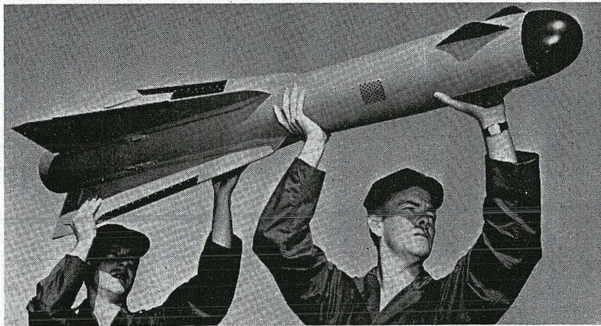
FALCON air-to-air missile, a guided aircraft rocket developed by Hughes Aircraft for the USAF. It's ability to manoeuvre is shown at left with a direct hit on a radio controlled B-17.
