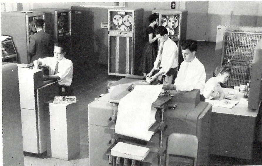
Avro's Computer Capacity was greatly increased with the addition, last year, of the IBM 704 electronic data processing machine shown above. Latest and most powerful digital computer available to industry, Avro's 704 is the only one outside the U.S. Staff of over 30 keep machine busy.
