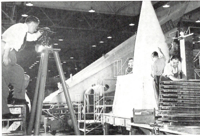
Transit is used to line up correct aerofoil forms of master models to horizontal and vertical datum lines. Work on these specially-fabricated tools began in mid-1954. Metal formers with plastic and plaster filler form tools.
