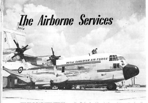
**FIRST RCAF HERCULES** to roll off the Lockheed (Georgia) production line is shown here. The Air Force, which has ordered four of the 60 ton transports, expects to put the first one in service by the end of this year. Hercules has four Allison T-56 turboprops, each rated at 4050 ehp for t/o.
