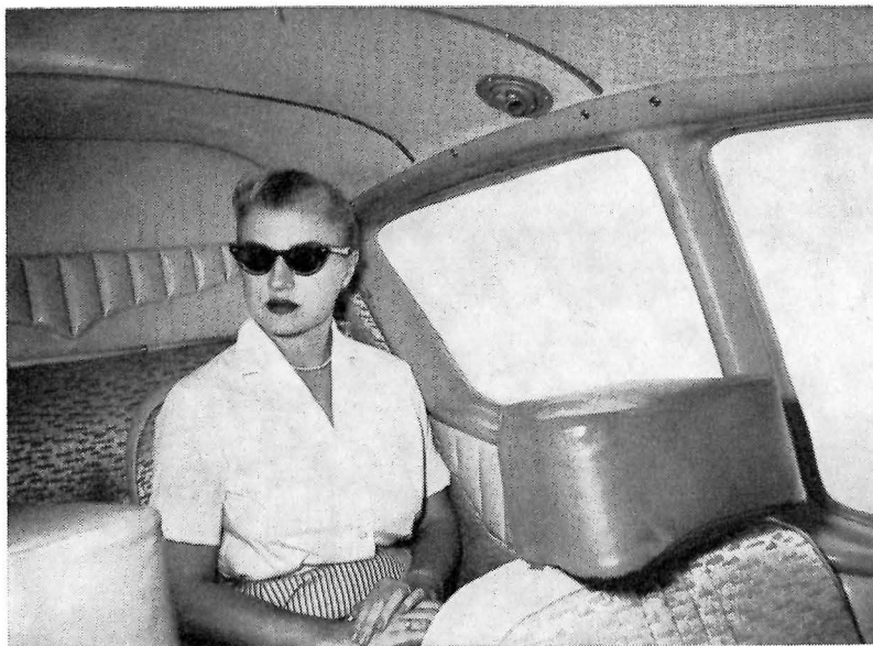
THIRD WINDOW FOR APACHE G: The new Piper Apache G features a full-size third window on each side aft. Windows afford better rearward vision for pilot as well as convenience for fifth seat passenger. Photo also shows striking new interior styling and newly designed headrests.
