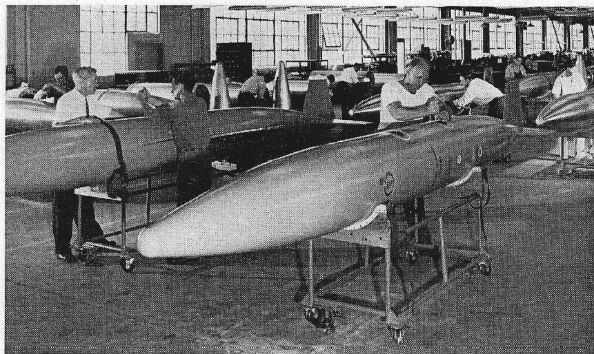
AVRO 104 PRODUCTION. CF-104 interceptor wing tip and pylon fuel tank production in progress at the Malton plant of Avro Aircraft Ltd. The company recently shipped the first of 300 sets of tanks manufactured under DDP contract, to Lockheed.
