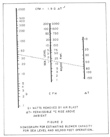
description of the second nomograph (Figure 2) which permits rapid selection of the maximum blower capacity required to meet the cooling needs. The basis for this chart is a constant pressure formula CFM  $\pm$  5.92 (T<sub>1</sub> + 273) Q.  $\triangle$  T which can be reduced to CFM = 1.9 Q.  $\triangle$  T cubic feet per minute where symbols have the same meaning as in figure (1). Using this chart, an adequate blower capacity may be selected for given heat and temperature rise conditions.
