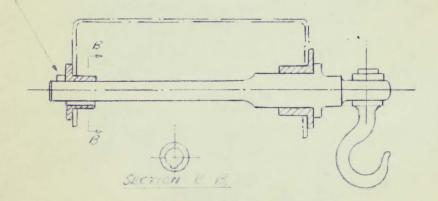
SECTION ON A SHOWING LIFTING BOOM
