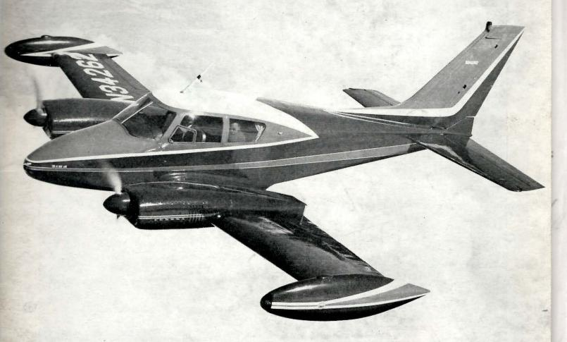
The 1960 look for the Cessna 310D features a new vertical fin which incorporates a 40° sweep. A non-congealing oil cooler has been added to the 310D's oil system.
