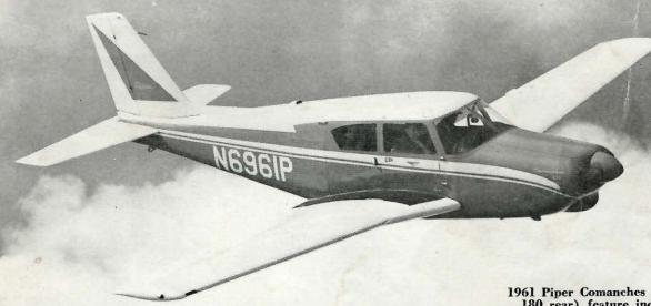
1961 Piper Comanches (250 front, 180 rear) feature increased fuel capacity for up to 1600 miles range, greater payload, new centrally controlled cabin ventilation system.
