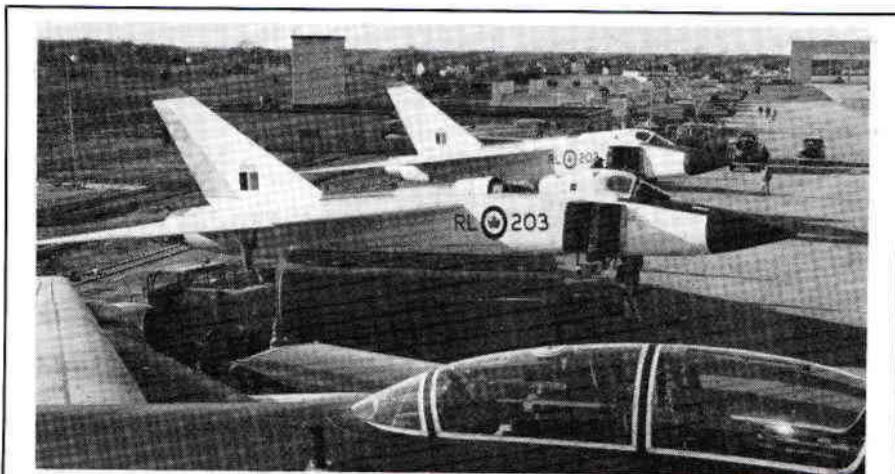
ARROWS ON FLIGHT LINE at Avro being prepared for flight test during vigorous development program. Arrow 203 in foreground—viewed over the cockpit of Orinda's B-47 Iroquois Test Bed—has its control surfaces highlighted with da-glo reflective paint.
