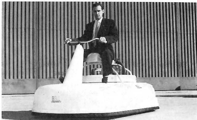
BELL AIR SCOOTER: Technically known as an air cushion vehicle, this new Bell machine is 30" high, 53" wide, 85" long and weighs 160 lbs. A 12-hp, 2 cycle motorscooter engine using a gas and oil mixture for fuel turns a fan of 30" diameter; the resulting air blast lifts the vehicle about two-and-one-half inches off the ground. Driver shifts his weight to turn and leans forward or back to go in either of those directions.
