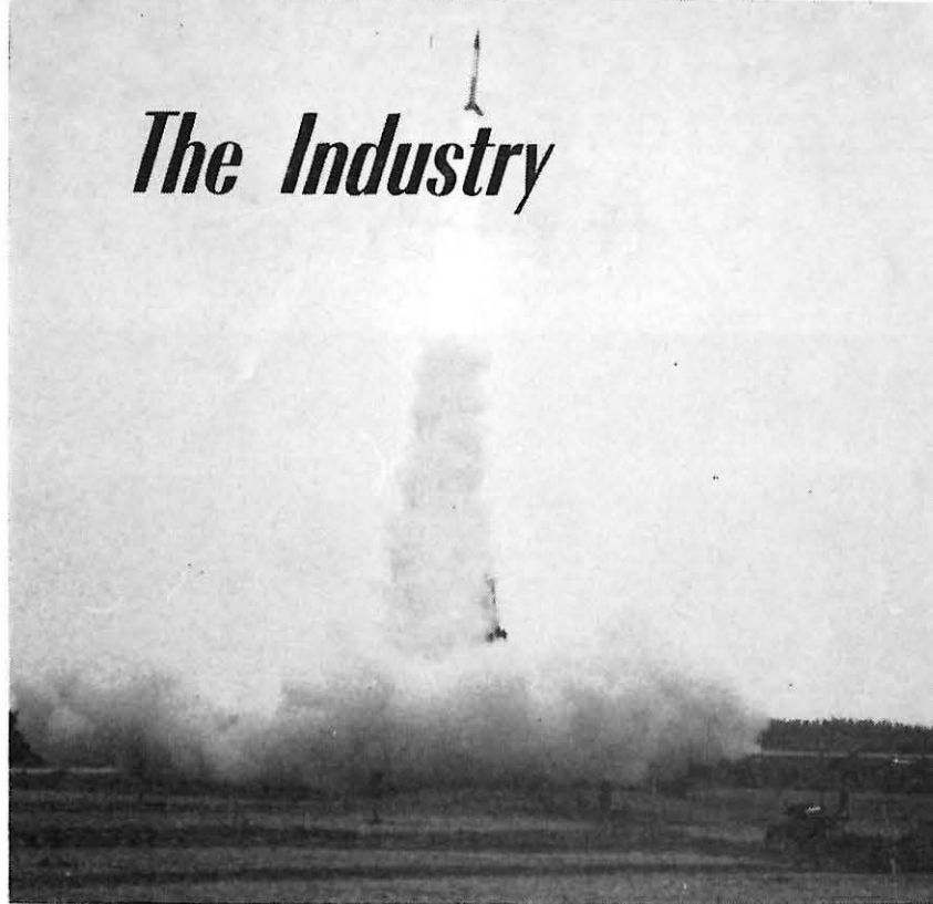
BLACK BRANT ROCKET , one of four launched by DRB from Churchill last September, gets away successfully. The 24-ft. propulsion test vehicles were developed by CARDE and were intended to test solid propellant fuels for use in future Canadian research rockets for upper atmospheric studies.
