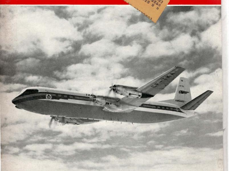
CF-TKA, first of 23 Vanguard 952's ordered by TCA, is currently engaged in C of A development flying. Powerplant for Vanguard 952 is 5545 ehp Rolls-Royce Tyne 11.
