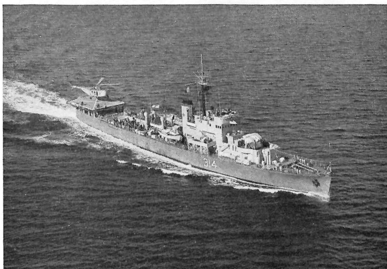
HELICOPTER PLATFORM: The RCN's HMCS Buckingham nests a Sikorsky on her newly constructed helicopter platform during trials being carried out to test the feasibility of operating helicopters from escort vessels. The Navy reports that no final assessment has been made as yet, but trials so far have been promising and further experimentation and evaluation of the scheme is planned.
