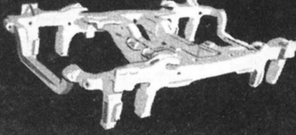
Truck frame for a railway coach cast in one piece by CSF.
