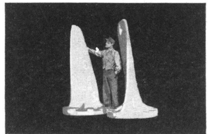
Marine propeller blades cast of nickel vanadium by CSF. Each blade weighs 3400 lbs.
