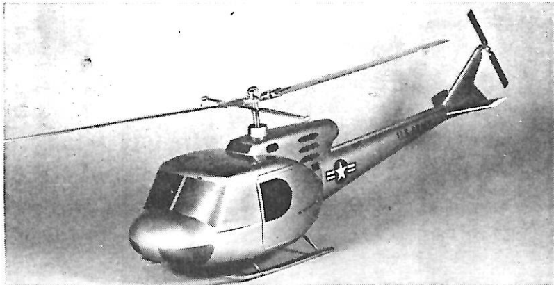
ANOTHER BELL: Model depicts the new Bell XH-40, now being developed by Bell Aircraft Corporation for the U.S. Army. To be powered by a new gas turbine engine, the Lycoming XT-53, the XH-40 is being designed primarily as a front line evacuation and instrument training aircraft. The new machine has a design cruising speed of over 100 knots and can carry more than 800 pounds of cargo. It is said to be somewhat larger than the 47 series machines. In its helicopter version, the new Lycoming engine is rated at 825 hp for military power and 770 hp for maximum continuous operation. XH-40 was winner of design competition in which all major helicopter companies participated.
