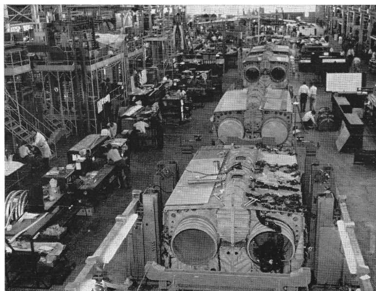
This general view of the Arrow Final Assembly shows major components being assembled for subsequent release to the final assembly marry-up in the background.
