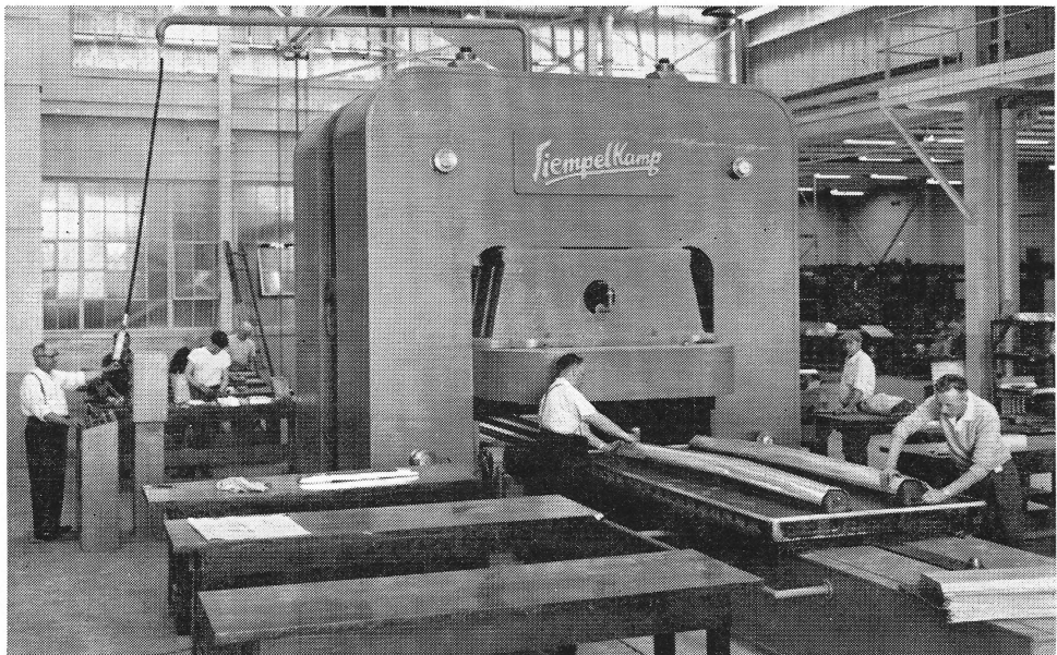
Largest rubber forming press in North America was installed for Arrow production. Able to form parts easily from heavier materials than previous needs, the pressure capacity is 15,000 tons.
