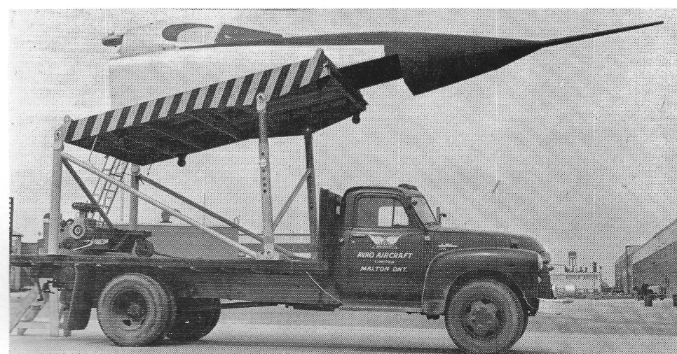
Mock-up of the cockpit was mounted on a truck at actual height and taxiing attitude of the Arrow in order to check pilot visibility under actual daylight and night operating conditions.
