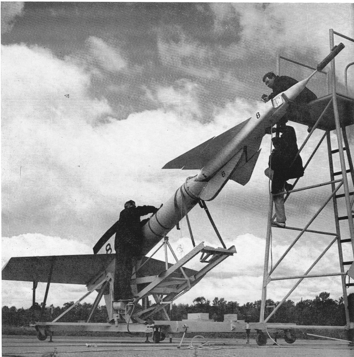
Large-scale Free-Flight Models were used in early development stages of the Arrow, to gather aerodynamic data. A model is seen here being readied on its launching rig with a Nike rocket booster in firing position.
