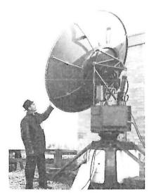
WEATHER RADAR actuators developed and produced by Found Bros. Aviation Ltd., have been added to four DoT-owned Decca MR-75 airport surveillance radars to convert them to weather radars. The Found Bros. actuator system tilts the rotating antenna at a rate of 1° per revolution. After 30 turns, antenna is returned to starting position.
