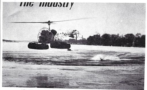
**AIR-TOWED SURVEY SOUNDER** developed by Edo (Canada) Ltd. is shown being demonstrated recently. The equipment, which can be towed by a Bell G2 at 30 kt., has been sold to the DoT and to the Dept. of Mines and Technical Surveys. Edo says further development could lead to military uses.
