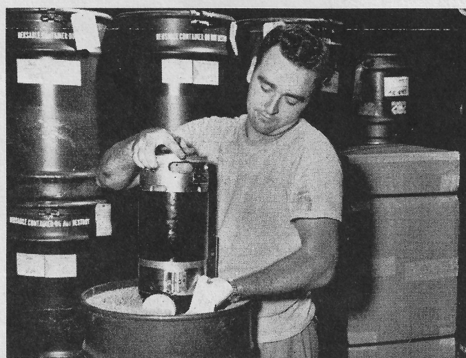
THIS IS PACKAGING DE-LUXE, and in the Part Departments it has become a science. Stowing an alternator in a specially designed canister for dry damage-free travel is Don Van Wyck. Parts are shipped wherever CF-100s are in service.
