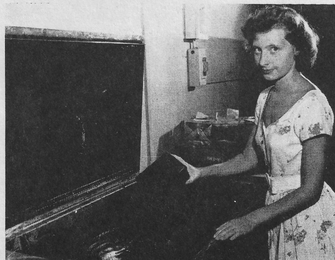
MOISTURE PLAYS HAVOC with stored parts unless they are well protected. To keep package free from moisture, Doreen Virtue dips it into bath of liquid wax which will harden into protective covering. Spares despatched: over 1,500,000 lbs to date.
