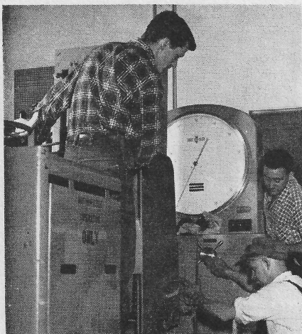
INSTALLING tensile machine in new Metallurgical laboratory are (from left): Bob Edwards, Ivan Daddson (kneeling) and Lee Morrison. Machine tests strength of metals under heat by tearing metal apart.
