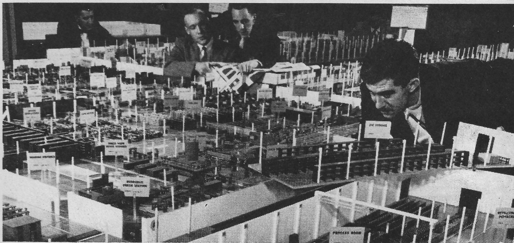
AVRO IN MINIATURE is seen here in the three-dimensional layout used to plan changes in production lines and facilities. A look at a new layout produces fast, clear picture for supervisors in shops where changes are to be made. From left: John Boardman, Dave Outram, Wally Walsh, Layout and Equipment Handling Supervisor, Len Morgan (rear) and Bob Martingell.
