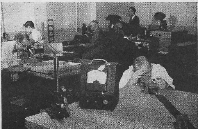
IN STANDARDS ROOM gauges used in the plant or let out to sub-contractors are checked to fractions of a thousandth part of an inch. In foreground working on surface plates are Howard Derouin (left), Cyril Moore. Room is kept at 68 deg.
