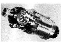
angles up to 60 degs in each direction can be obtained and the nosewheel can be turned through 360 degs for ground handling without mechanical disconnection. Canada: Dowty Equipment of Canada Ltd., Ajax, Ont.
