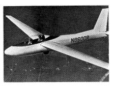
N.Y. Greater attention to pilot and passenger comfort has been afforded while maintaining safety factors. Designated the 2-32, it has roomy cockpit, high visibility, and a 500 lb useful load; can be used to carry two passengers in addition to the pilot, but retains a relatively high performance.
