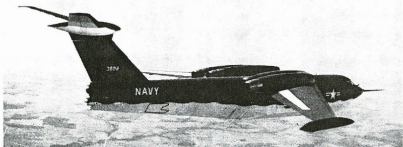
P6M MARTIN SEAMASTER: With an operational cruise altitude of 40,000 feet, the US Navy's SeaMaster is capable of high speeds at low levels to perform its mine-laying or photo-reconnaissance work. The P6M is shown below during taxi trials on Chesapeake Bay. Note canted engine nacelles to prevent afterbody heating.
