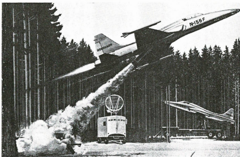
ZERO-LAUNCH FIGHTER: Shown is an artist's conception of the Northrop N-156F supersonic fighter being launched from small, hidden forest clearing. The lightweight fighter is being developed for use by NATO nations. Zero-launch capability is based on use of launchers presently available. The missile-carrying N-156F is capable of Mach 2; can be operated from short airstrips and grass fields.
