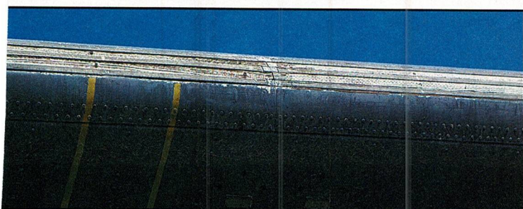
Laminated wood leading edges serve as de-icing devices.
